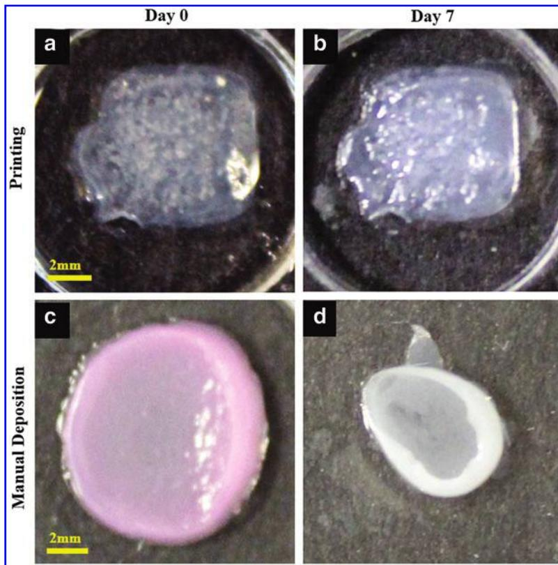
**FIG. 6.** Shape and form of printed skin tissue. A comparison of skin tissues fabricated via 3D bioprinting and manual deposition indicates that printed skin samples (**a**, **b**) retain their form (dimensions) and shape, whereas manually deposited structures (**c**, **d**) shrink and form concave shapes (buckle) under submerged culture condition after 7 days. Color images available online at [www.liebertpub.com/tec](http://www.liebertpub.com/tec)
