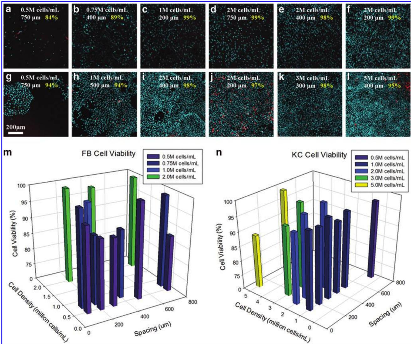
**FIG. 3.** Optimization of printing parameters for individual cell cultures. Cell suspension density and resolution (spacing between droplets) were varied over a broad range for FBs (a–f) and keratinocytes (KCs) (g–l) printed in monolayers. Cell viability was assessed at each condition after 7 days in culture (m, n). Color images available online at [www.liebertpub.com/tec](http://www.liebertpub.com/tec)
